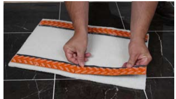
Example of how to mount diamonds to driver pad
